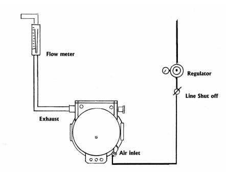
The minimum acceptable flow rate for a new Air Hat is 12 cfm. The average cfm reading for new Air Hats has fallen between 15–18 cfm. The most common fault for not reaching 12 cfm is over packing the air diffuser with Lambswool. Any failure to reach 12 cfm should be investigated.
