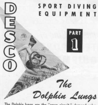
The Dolphin lungs are the "open circuit," demand valve type using compressed air. The demand valve is placed on the DESCO U. S. Navy type full face mask, and operates at 70 p.s.i. supplied by a pre-set regulator located on the lung backboard. The chrome demand valve allows effortless breathing at any depth and is fully automatic. A "free flow button" is provided on the valve to furnish a direct flow of air at the touch of a finger.
